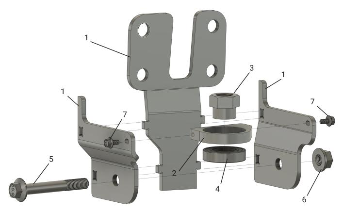
Note: Track bar reinforcement bracket is supplied fully welded as a single piece. Exploded diagram for clarity.
