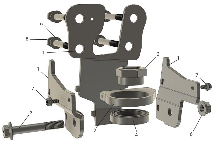
Note: Track bar reinforcement bracket is supplied fully welded as a single piece. Exploded diagram for clarity.
